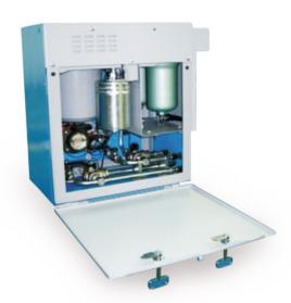
Meter MD-K1 type is designed for precise measurement of fuel consumption by diesel engine a8VC22 type SM 42 locomotive.
