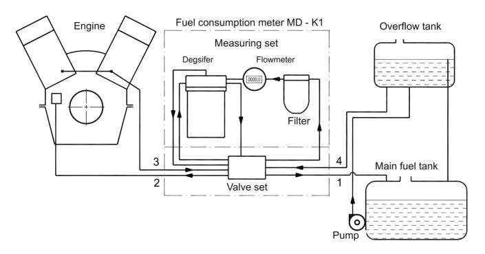
The measurement of flow rate is realized by volume flowmeters.
